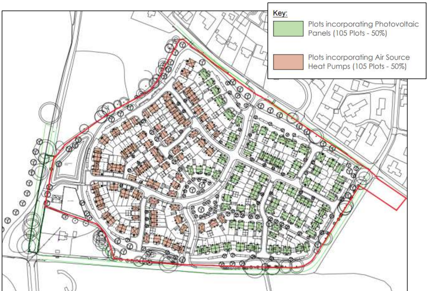
figure 22: PV and air source heat pump distribution
